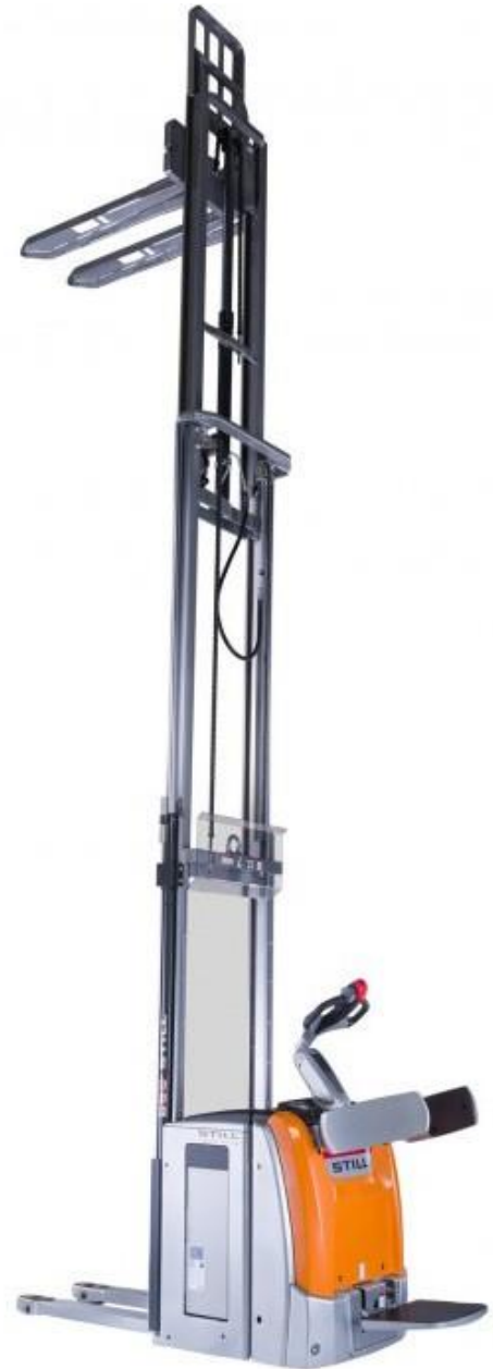
triplex mast with 2 extendible sections
