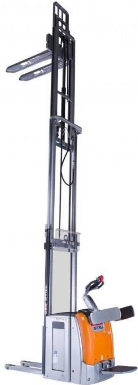
triplex mast with 2 extendible sections
